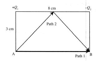
34. A particle with charge +q is moved from point A to point B along Path 1 in the picture above and experiences a change in potential energy given by  $\Delta U$ . What would the change in potential energy be if the charge had the opposite sign and moved along Path 2 from point A to point B instead of along Path 1?
